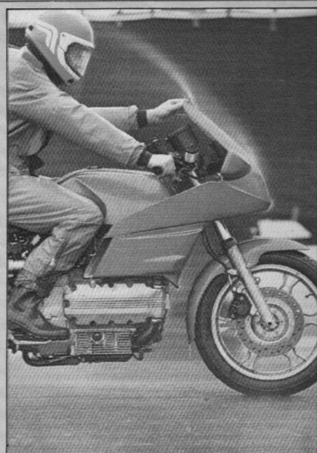
Above: wind tunnel development of the faired version produced this adjustable spoiler.
